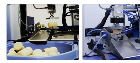
Testing the elastic properties of all types of cylindrical, straight cork stoppers is a key parameter in selecting their suitability for different wines and spirits. Good resilience enhances good corking impermeability.
